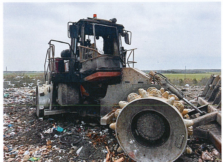
Compactor after fire extinguished
